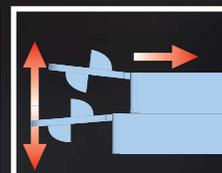
*To open, insert finger between two locking tabs and slide back upper UniMailer™.*
