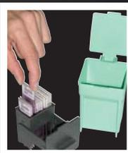
Vertical rack eases slide removal without using forceps.
