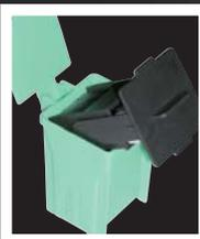
Staining rack is placed at an angle to facilitate draining of slides.
