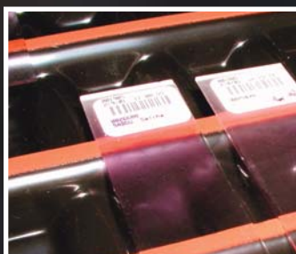
Wells between rails can be used to hold water for techniques needing a humid environment.
